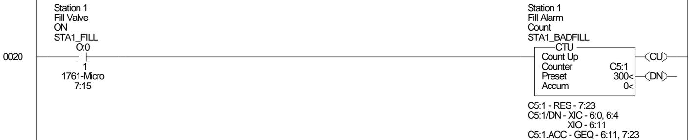
This is how long the level switch must show full before the 'bad fill' counter is reset.
