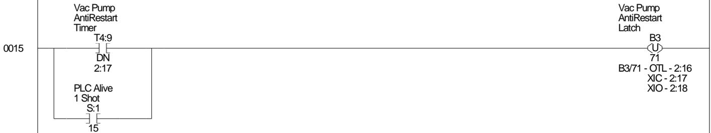
The moment the vac pump turns off, and there isn't a call for fill then one shot on this latch relay, which is then timed out for the setpoint in the 'Vac Pump Antirestart' timer. This prevents the pump from short cycling.
