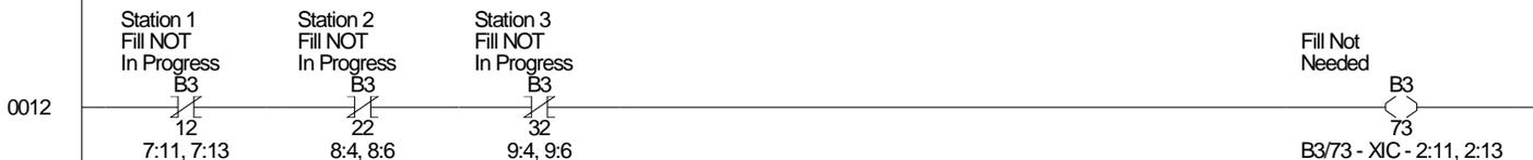
Unlatch the call for vac upon initialization, and when no station is calling for material.
