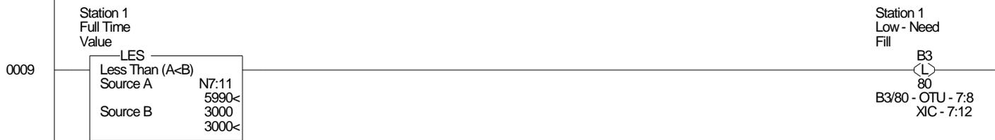
This retentive timer is reset once per minute, so can time out to a maximum value of 6000. Greater and less than comparisons are performed using the accumulated value at the one minute mark to determine whether Station 1 is below or above the high level sensor. Note: because it is evaluated only once per minute it will normally allow a load one cycle past the point where the low level pilot lamp turns off.
