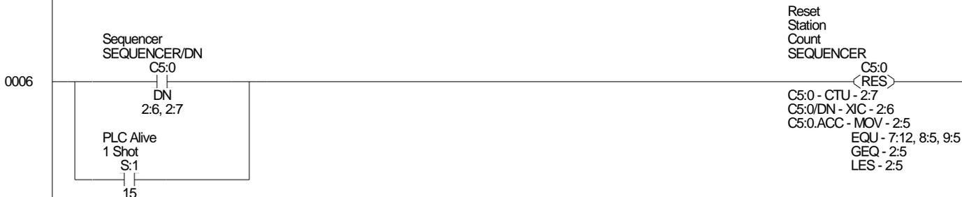
This is the core rung of the station selection logic. The count increments cyclically and pauses when it encounters a station with a fill in progress. When the fill completes cycling resumes.
