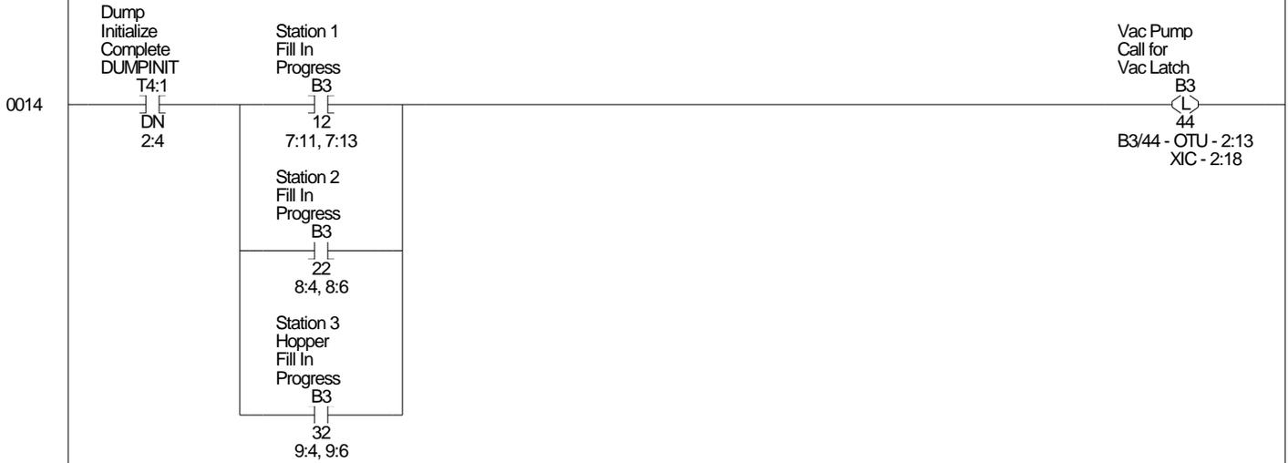
After the anti-restart timer finishes, and the DN (done) bit is set the next call for material will unlatch the anti-restart bit, and allow the vac pump to turn on again.
