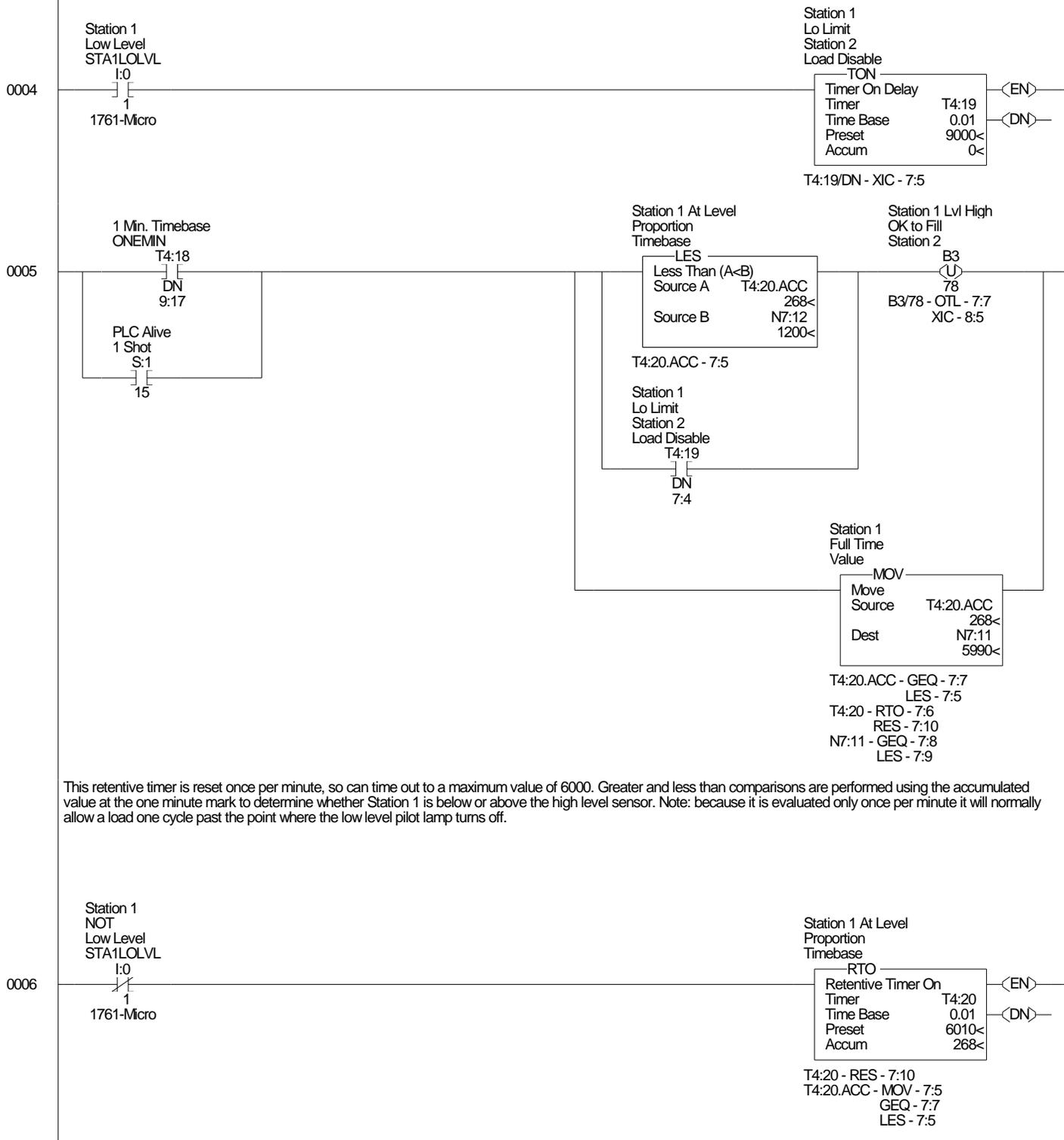
These rungs are a crude proportioning device to show station 1 fill level. The high level sensor is fed into a retentive timer, and the accumulated time is evaluated every minute. If the full time is more than 50% then station 1 is considered full, and if less than 30% considered empty. The proportioning values aren't programic, and can be changed by altering the N7 registers to other values.
