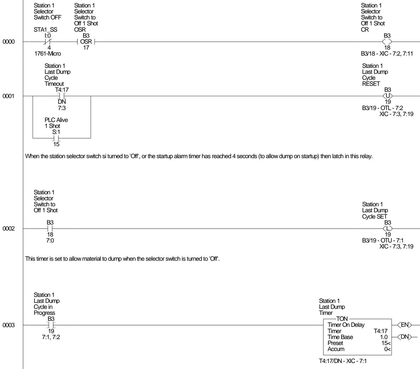
Station 1 - Allow Dryer Load Level Determination
