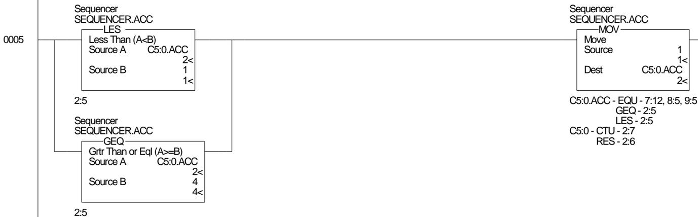
If the counter ever goes to some wierd value, then plonk it back down to station 1 by resetting the counter.
