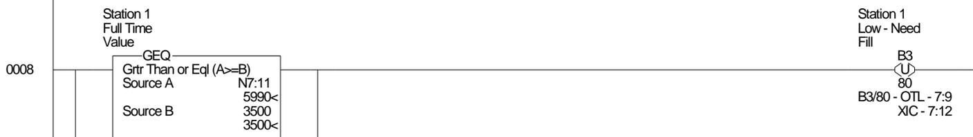
If station 1 level is high for less than half the time (3000 of 6000 - 30 in 60 seconds) then consider it low.
