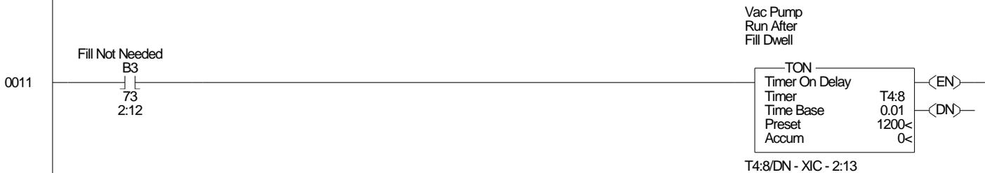
When no stations have called to be filled turn on this bit. It is used to control vacuum loader operation.
