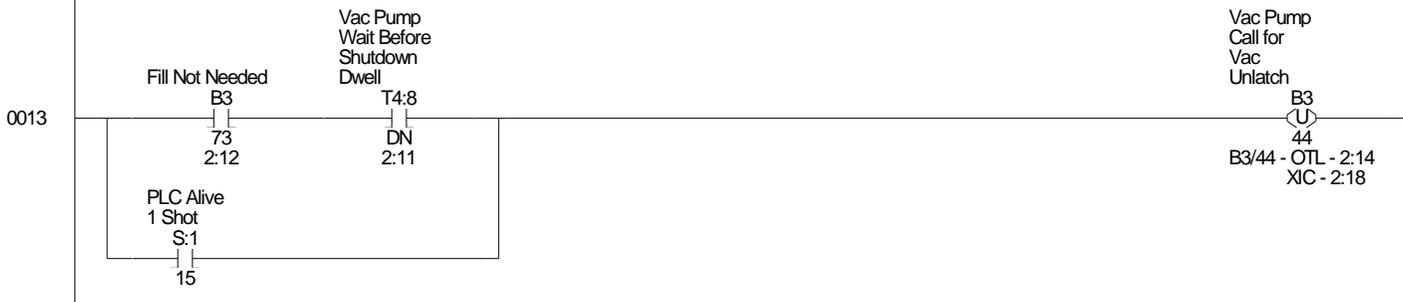
After dump initialize completes on startup, the vac pump run status is controlled by the stations as they call for fill. If the motor auxiliary does not close the circuit within T4:7 after a call for motor start then a fault will occur.
