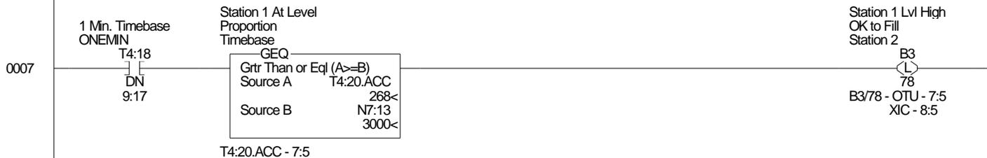
If station 1 level is high for less than half the time (3000 of 6000 - 30 in 60 seconds) then consider it low.
