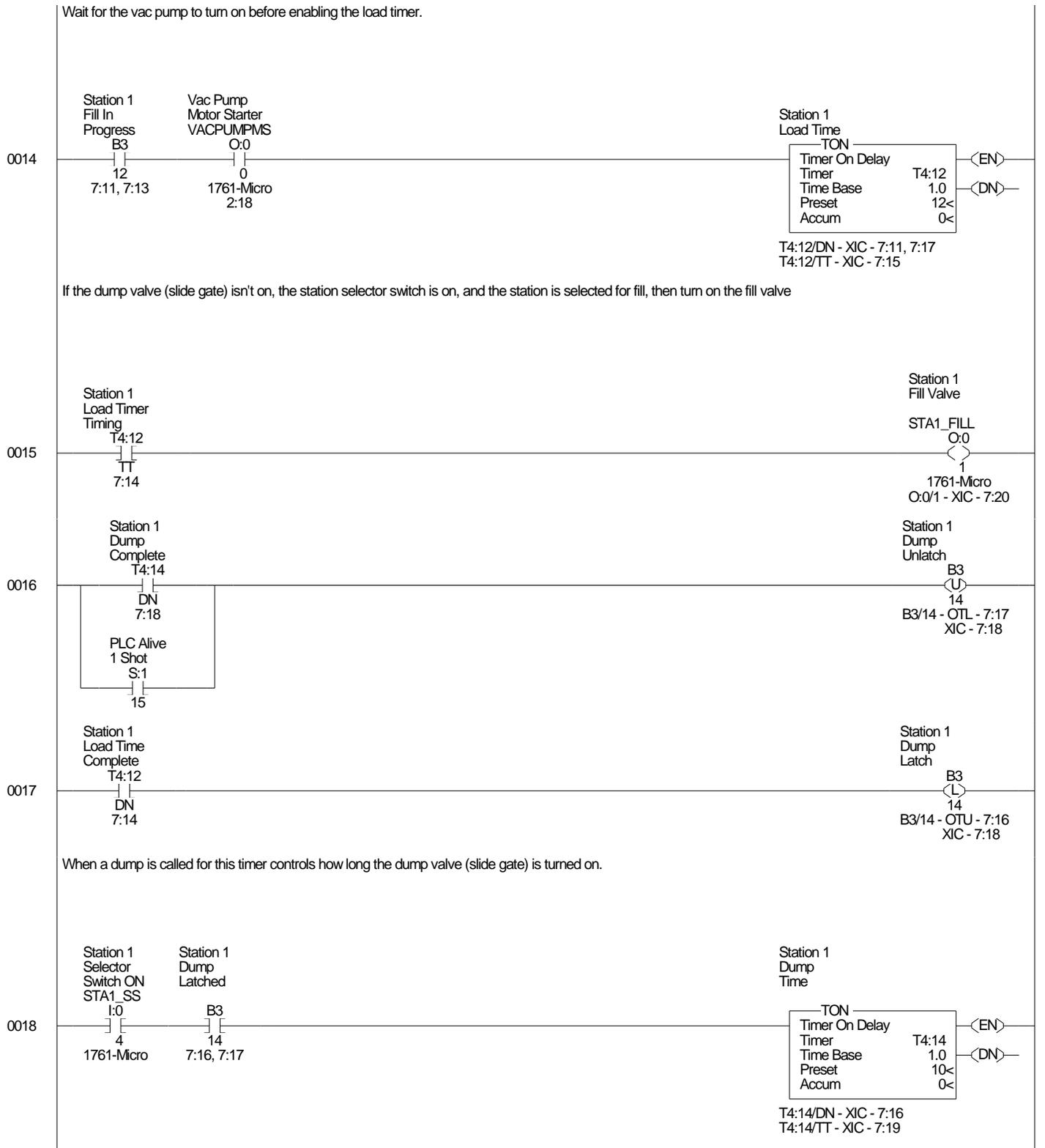
The dump valve (slide gate) is turned on during normal operation in the first line of this rung, when the selector switch is turned to 'Off' (for one last cycle) in the second line, and during system initialization in the third line.
