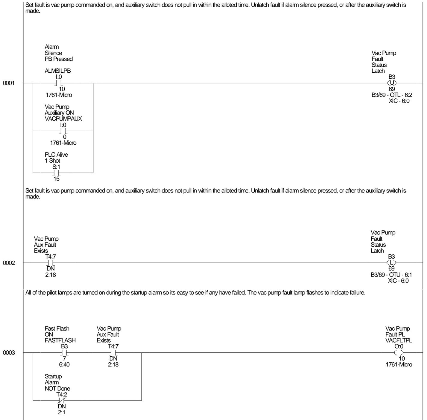
Slow flash for an early warning of poor filling performance, and turn on 100% for load failure.
